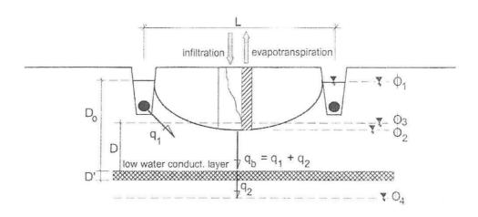
Fig. 1. Physical concept of the SWATREZ model
